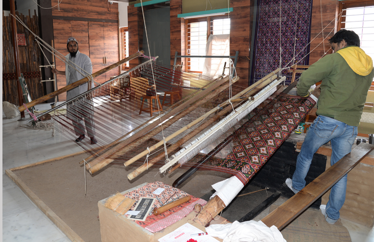
Figure 5.36h Winding the cloth beam of the suspended loom at Patan Patola Heritage, Gujarat, India (photograph by Carol Ventura, 2016).
