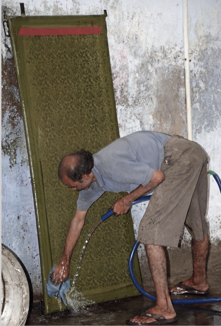
Figure 5.34d Washing the screen after printing in Ahmedabad, India (photograph by Carol Ventura, 2016).
