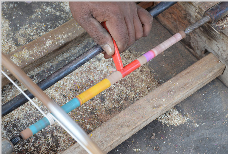
Figure 5.25e Applying lacquer to wood rotating on a bow lathe in Nirona, Kutch, Gujarat, India (photograph by Carol Ventura, 2016).
