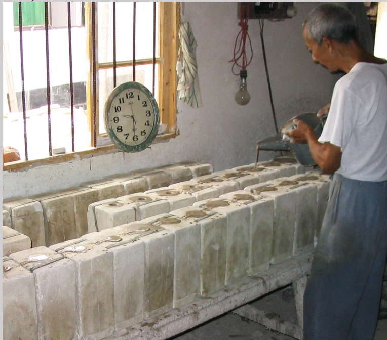
Figure 5.13a Filling plaster molds with porcelain slip in Jingdezhen, China (photograph by Carol Ventura, 2004).
