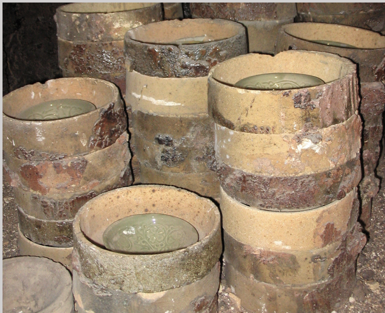
5.15b Saggars with celadon-glazed porcelain bowls in the Shanghai Museum, China (photograph by Carol Ventura, 2004).
