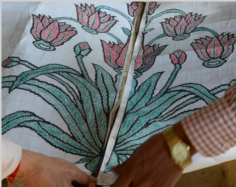
Figure 5.38i Paper graph for the voided velvet fabric on the drawloom in Cholapur, India (photograph by Carol Ventura, 2016).
