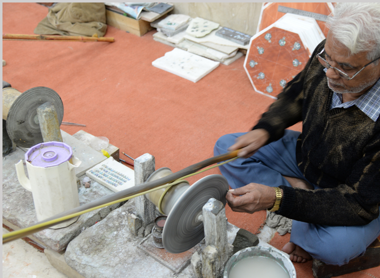
Figure 5.39d Shaping stone inlay piece against a rotating abrasive wheel turned with a bow in Agra, India (photograph by Carol Ventura, 2016).
