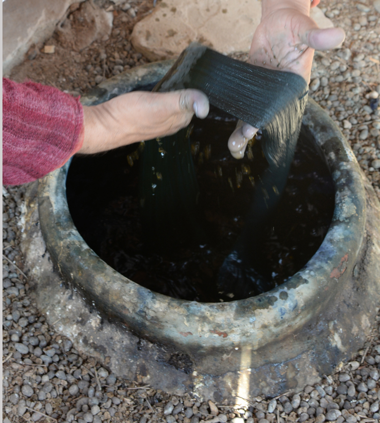
Figure 5.29a Shamji Vankar rotates a wool skein into a partially buried ceramic indigo vat. The yarn emerges green but turns blue as it absorbs oxygen in Bhujodi, India (photograph by Carol Ventura, 2016).
