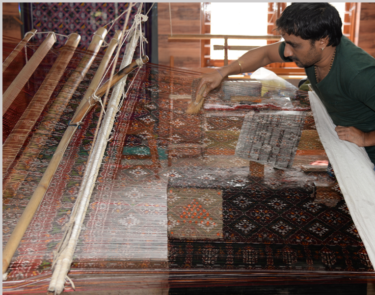
Figure 5.36n Rahulbhai Salvi spreads the sizing with a brush to strengthen the delicate tie-dyed silk threads in Patan, Gujarat, India (photograph by Carol Ventura, 2016).
