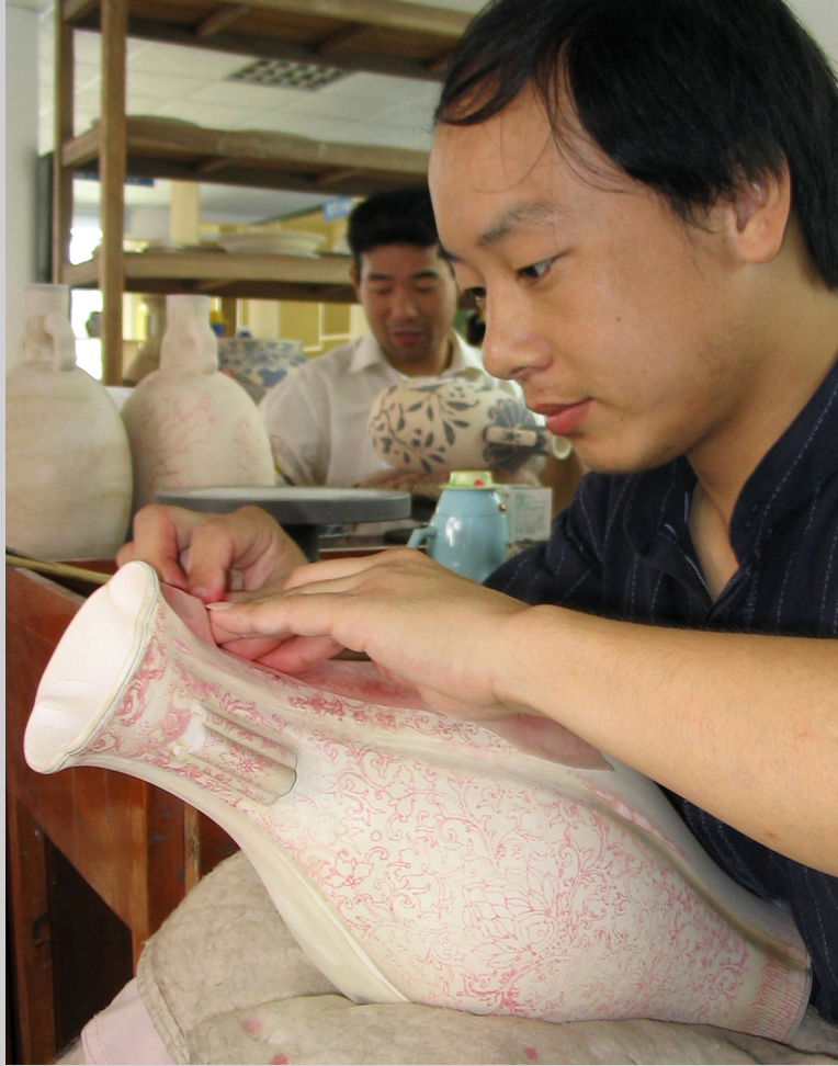
Figure 5.14a A stencil is used to transfer the pattern onto greenware at the Jiayang Ceramics Company in Jingdezhen, China (photograph by Carol Ventura, 2004).
