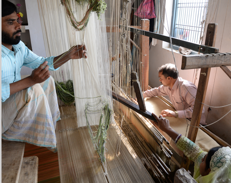
Figure 5.38b While Belal selects drawcords for the next pattern shed, Rijvana Ansari inserts an angle hook that helps separate the cords, and her husband, Shamin, weaves the silk ground twill with foot treadles on their drawloom in Cholapur, India (photograph by Carol Ventura, 2016).
