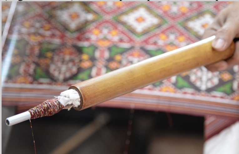
Figure 5.36i Shuttle with bobbin of dyed weft at Patan Patola Heritage, Gujarat, India (photograph by Carol Ventura, 2016).
