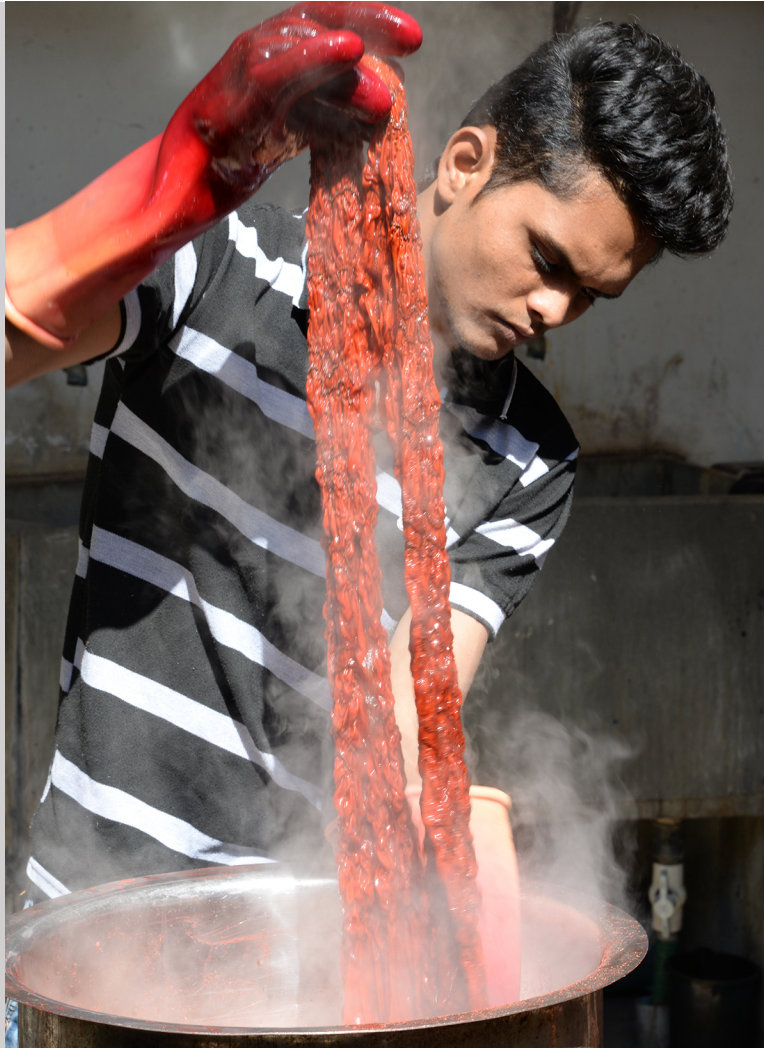
Figure 5.31e The wrapped cloth is dipped in and out of hot dye, then hung to dry at Sidr Craft in Bjuh, Gujarat, India (photograph by Carol Ventura, 2016).
