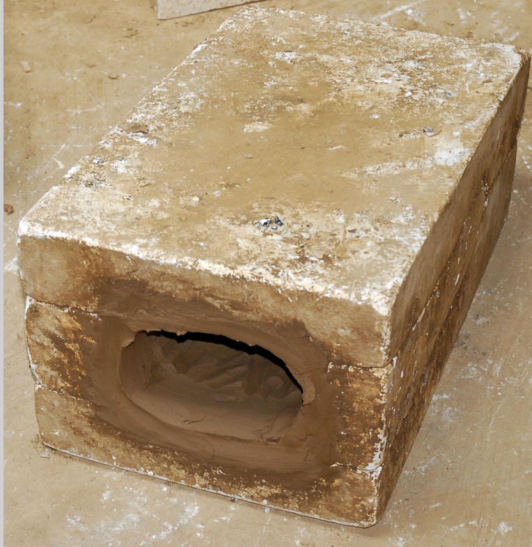
Figure 5.6c The mold is put together, then opened when the clay has dried enough to keep its form at the Art Ceramics and Lacquer Factory, Xian, China (photograph by Carol Ventura, 2013).
