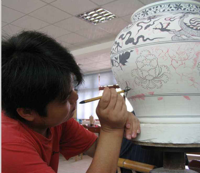
Figure 5.14b Cobalt underglaze is painted over the stenciled lines, which will burn off during firing at the Jiayang Ceramics Company in Jingdezhen, China (photograph by Carol Ventura, 2004).
