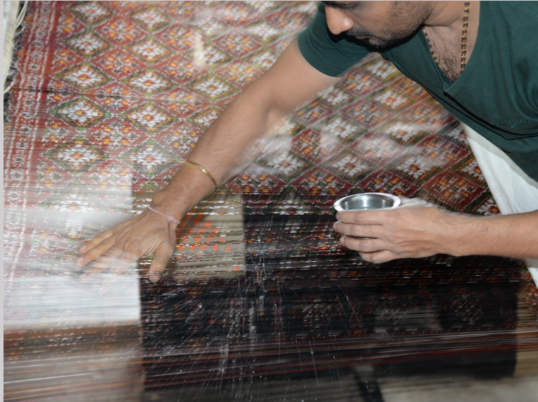
Figure 5.36m Rahulbhai Salvi applies rice water sizing to the unwoven tie-dyed silk warp with his hand in Patan, Gujarat, India (photograph by Carol Ventura, 2016).
