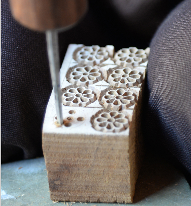
Figure 5.32d A sharp metal bit cuts holes as it is rotated in a block of wood at the Anokhi Museum of Hand Printing, Jaipur, India (photograph by Carol Ventura, 2016).
