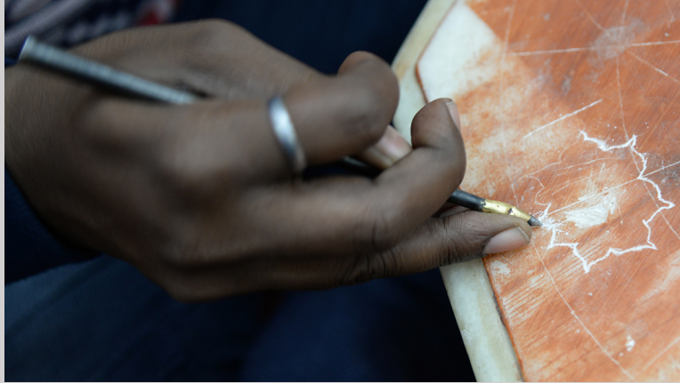
Figure 5.39c Carving a stone matrix for inlay in Agra, India (photograph by Carol Ventura, 2016).
