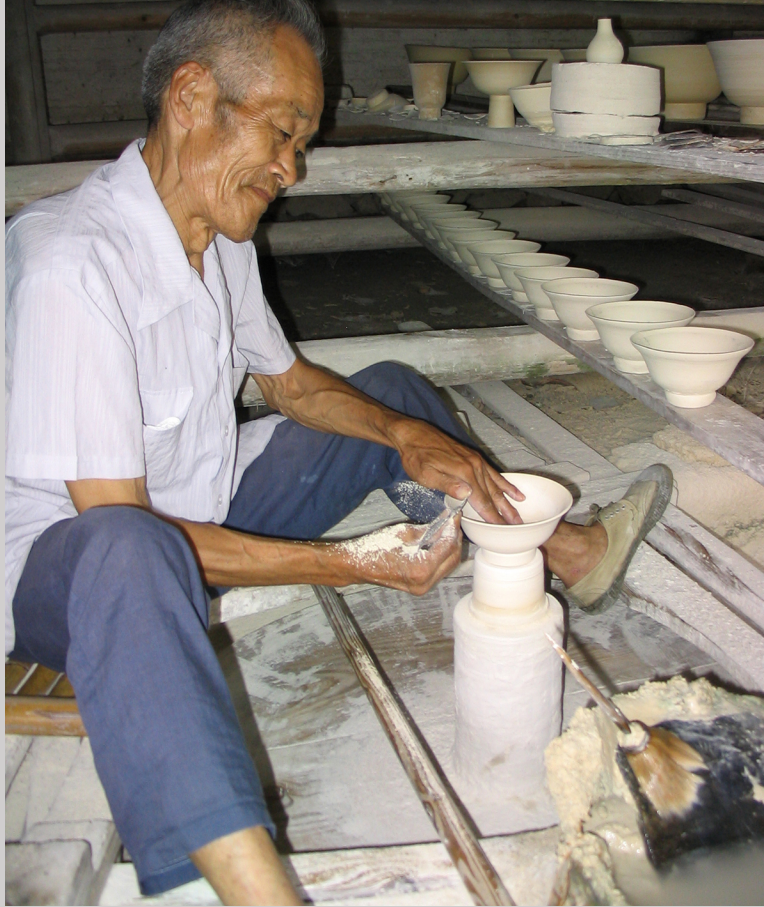
Figure 5.12c The walls of the piece are then trimmed to make them thinner at the Jingdezhen Ceramic History Museum, China (photograph by Carol Ventura, 2004).
