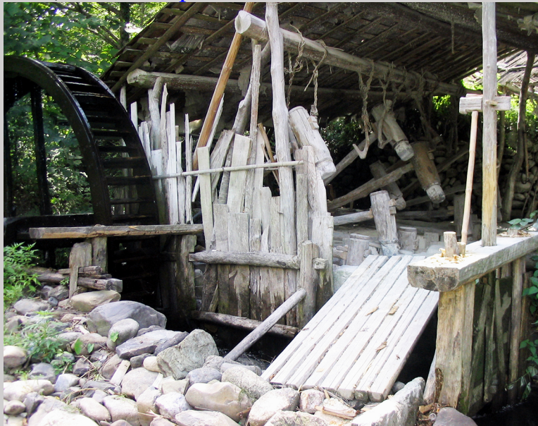
5.11a China stone is quarried nearby, broken into pieces, then ground into a fine powder with water-powered trip-hammers in Yaoli, China (photograph by Carol Ventura, 2004).
