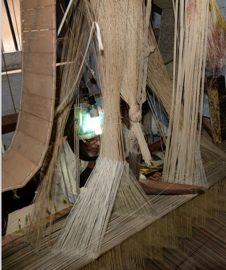
Figure 5.38n Strung together punched cards (on the left) control the sheds in place of the cut cords on this jacquard loom that was converted from a drawloom in Varanasi, India (photograph by Carol Ventura, 2016).
