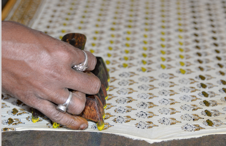
Figure 5.32k Block printing yellow on stretched cotton in Bagru, Jaipur, India (photograph by Carol Ventura, 2016).
