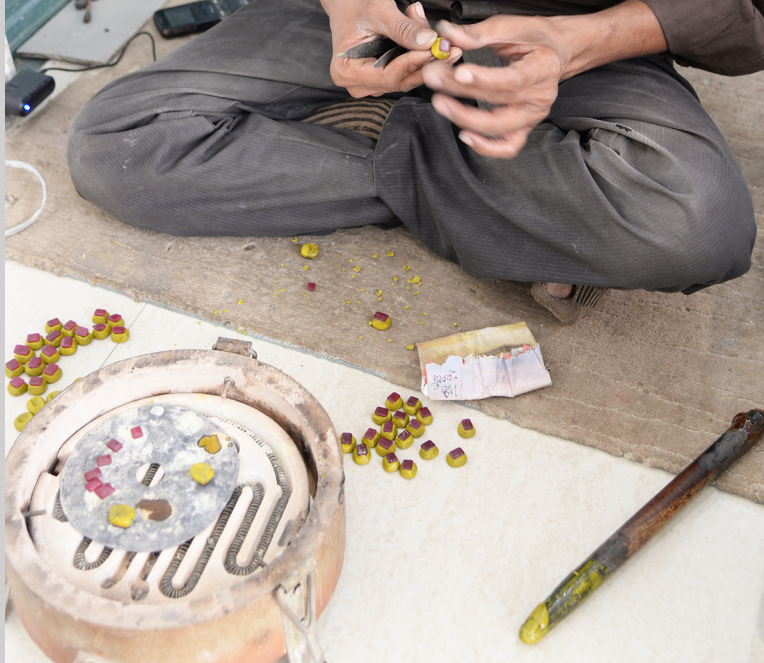
Figure 5.39e Attaching warm dopping wax to stones in Jaipur, India (photograph by Carol Ventura, 2016).
