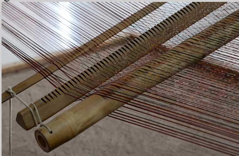
Figure 5.36g A grooved warp spreader keeps the patterned warps evenly spaced while weaving on the loom at Patan Patola Heritage, Gujarat, India (photograph by Carol Ventura, 2016).
