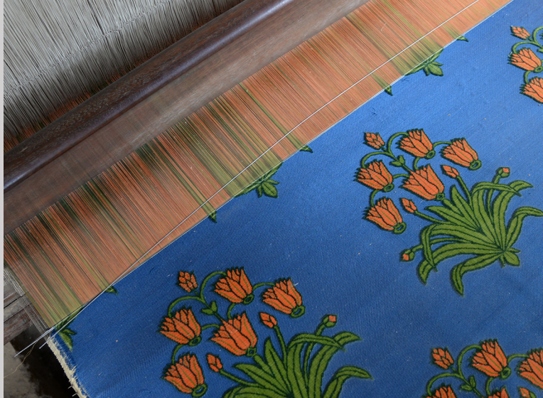
Figure 5.38j Woven voided velvet silk fabric on the drawloom in Cholapur, India (photograph by Carol Ventura, 2016).
