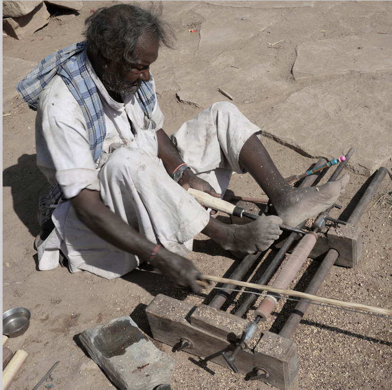
Figure 5.25a Bhachaya moves a bow back and forth with his right hand while operating a cutting tool with his left and his right foot to turn wood on a bow lathe in Nirona, Kutch, Gujarat, India (photograph by Carol Ventura, 2016).
