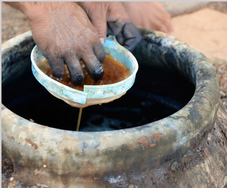
Figure 5.29e The indigo vat is fed fructose to keep the dye active in Bhujodi, India (photographs by Carol Ventura, 2016).
