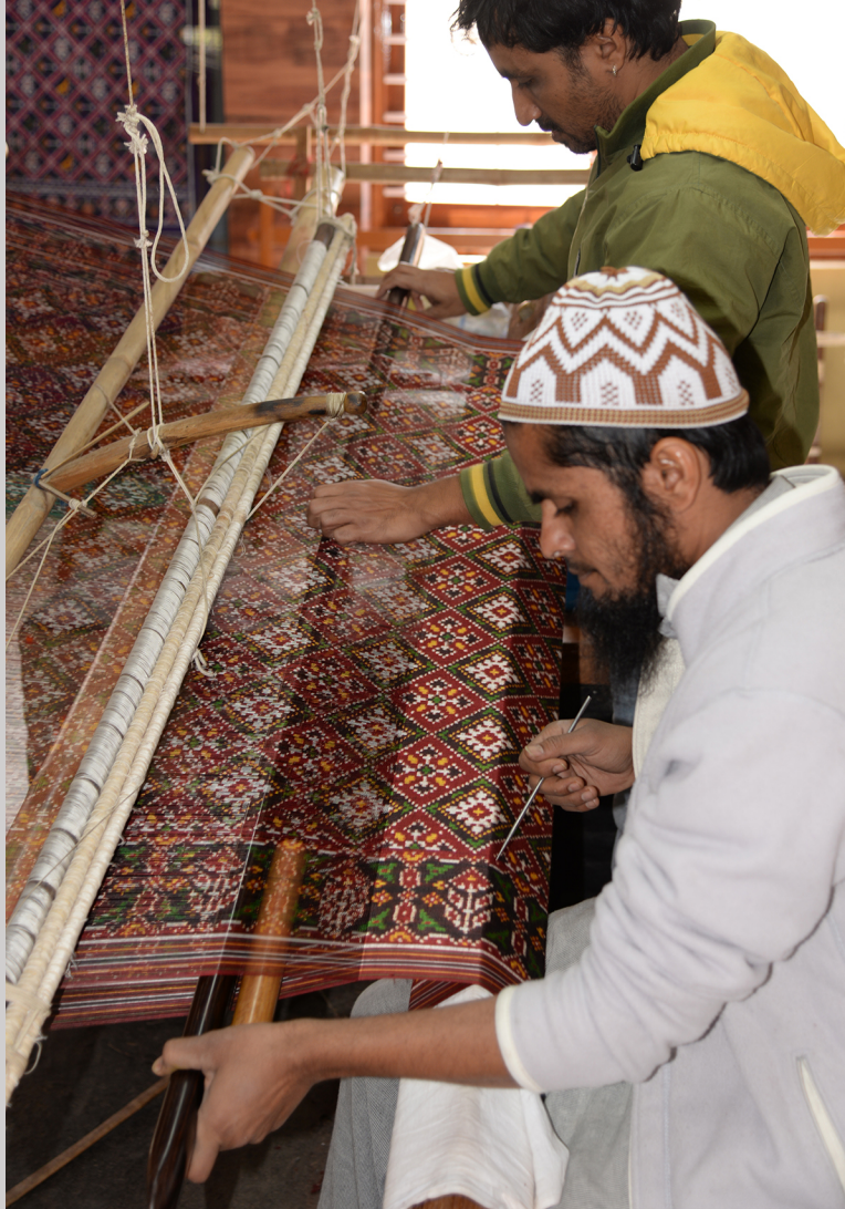
Figure 5.36j Inserting a shuttle of weft with the left hand while adjusting the placement of the threads with the right at Patan Patola Heritage, Gujarat, India (photograph by Carol Ventura, 2016).
