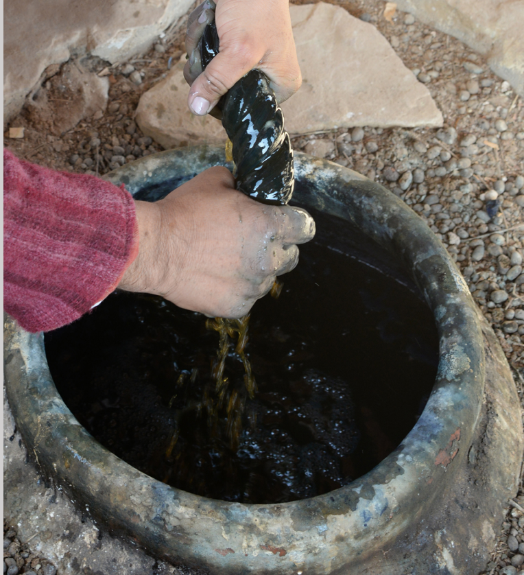
Figure 5.29b Shamji Vankar wrings the wool that was dipped into the indigo vat in Bhujodi, India (photograph by Carol Ventura, 2016).
