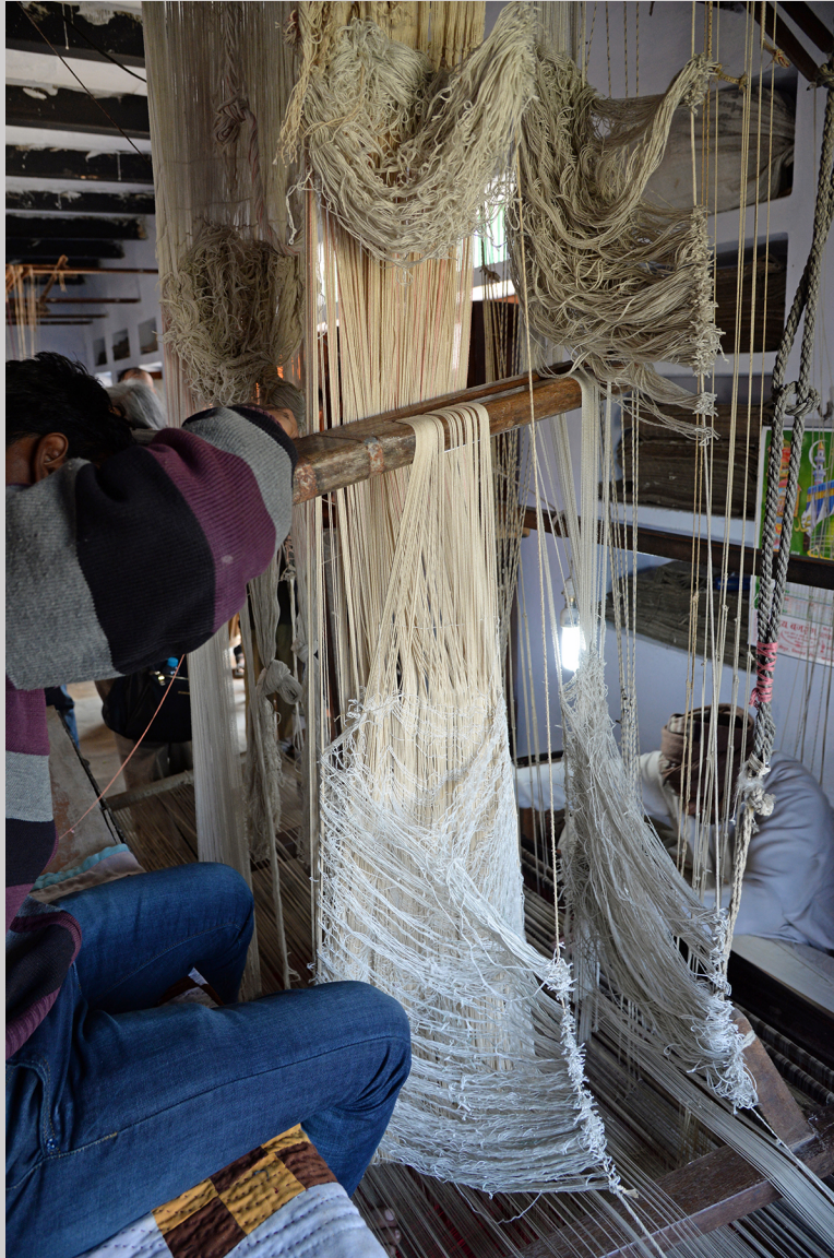
Figure 5.37b A “draw boy” uses a lifting fork to raise the appropriate drawcords to lift the harnesses in Cholapur, India (photograph by Carol Ventura, 2016).
