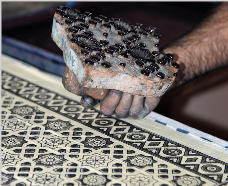
Figure 5.32h A dye-loaded wooden block ready to print at Dr. Ismail Mohmed Khatri Workshop in Bhuj, Gujarat, India (photograph by Carol Ventura, 2016).
