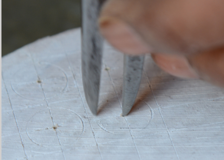
Figure 5.32b Marking a block to be cut at the Anokhi Museum of Hand Printing, Jaipur, India (photograph by Carol Ventura, 2016).
