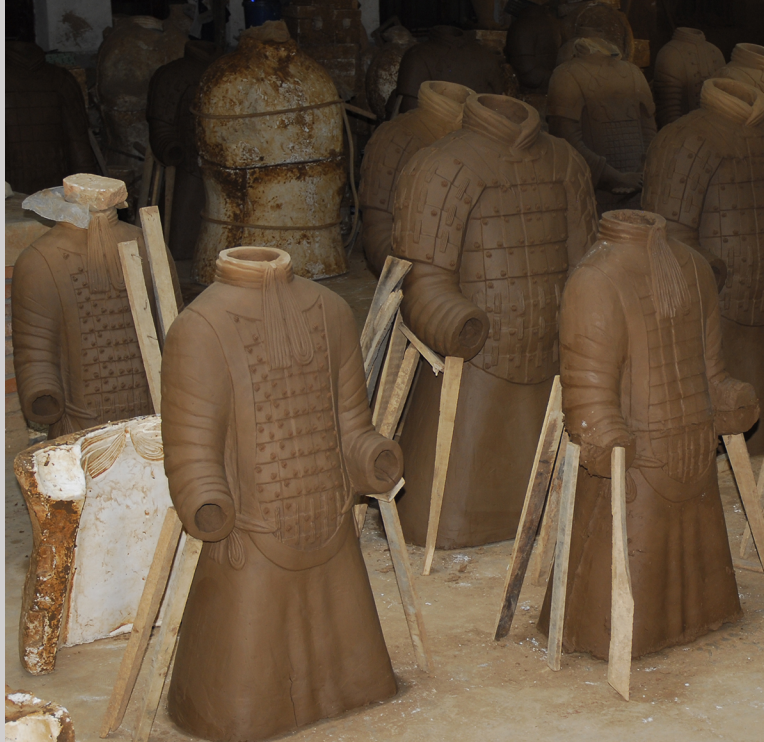
Figure 5.6d Leather-hard pieces are removed from molds and overhanging parts are supported as they dry at the Art Ceramics and Lacquer Factory, Xian, China (photograph by Carol Ventura, 2013).
