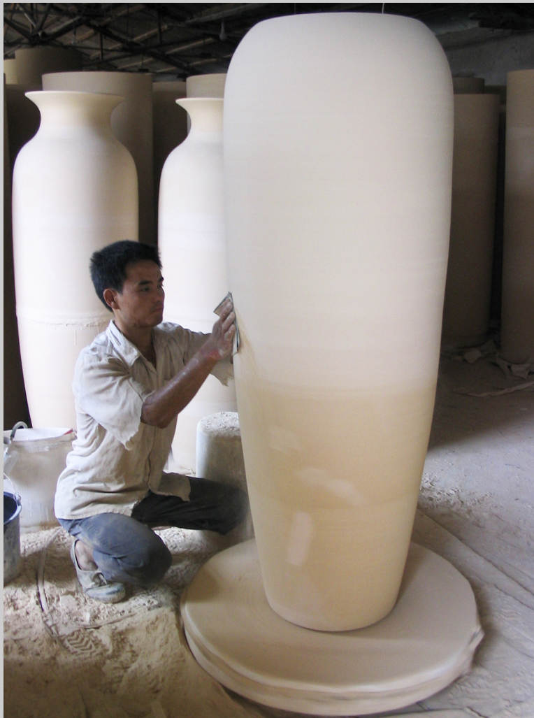
Figure 5.12i A pot is trimmed in the foreground, while clay is prepared for throwing in the middle ground and centered in the background at IAPFH in Jingdezhen, China (photograph by Carol Ventura, 2004).
