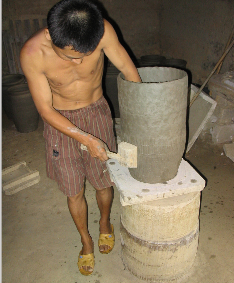
Figure 5.8b He textures the sides of the piece with a wooden paddle in Tianbao, China (photograph by Carol Ventura, 2004).
