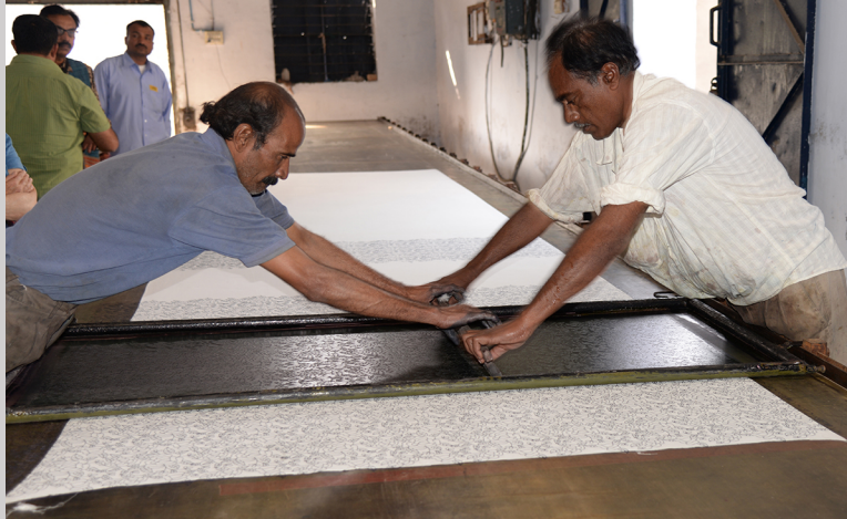
Figure 5.34b The screen is attached to a rail on one side to help with registration as it is moved across the cotton cloth during printing in Ahmedabad, India (photograph by Carol Ventura, 2016).
