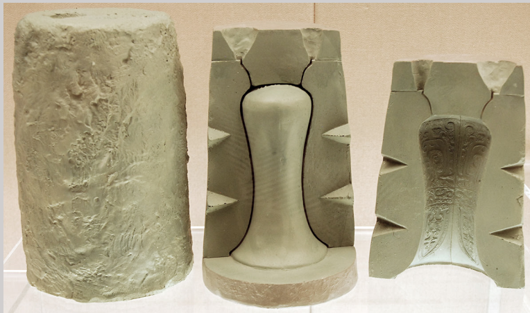
Figure 5.3b Closed and open three-piece clay mold used to cast a bronze vessel (photograph by Carol Ventura, Shanghai Museum, 2013).
