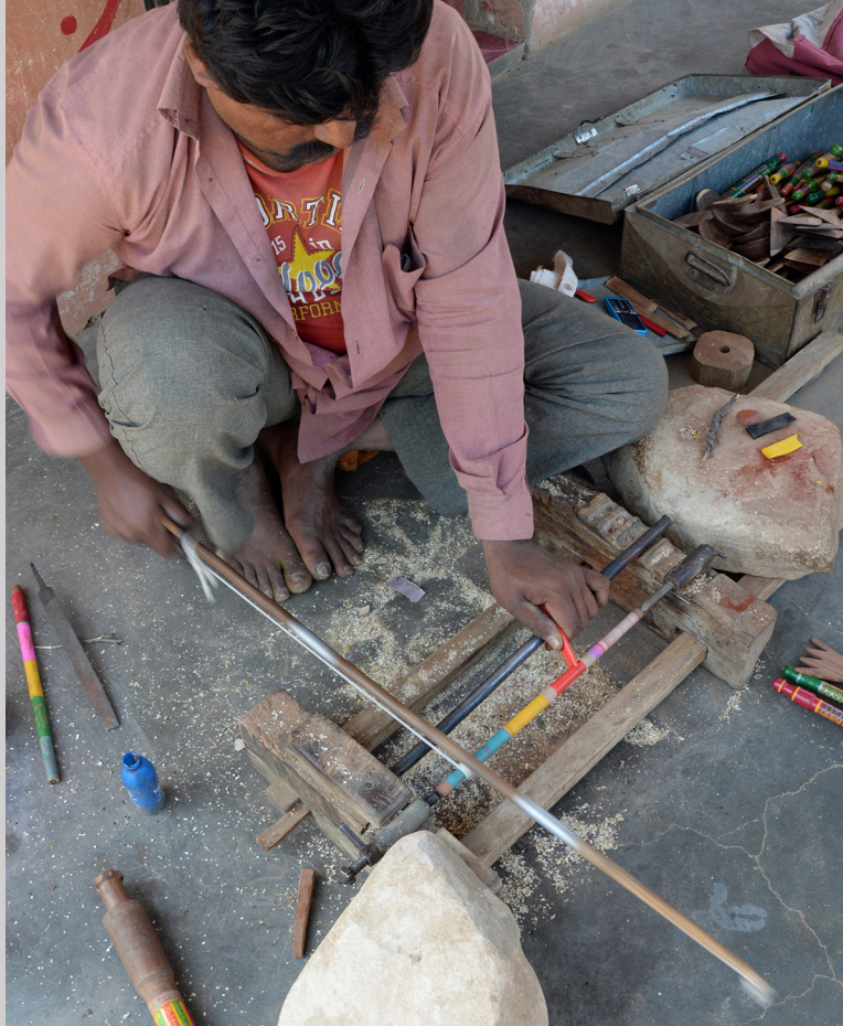
Figure 5.25d Applying lacquer to wood rotating on a bow lathe in Nirona, Kutch, Gujarat, India (photograph by Carol Ventura, 2016).
