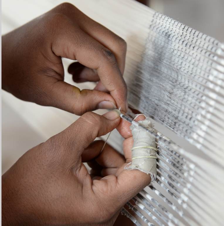
Figure 5.36c Bundles of threads were marked then the parts that are to remain white are tightly wrapped to stop dye from penetrating at Patan Patola Heritage, Gujarat, India (photograph by Carol Ventura, 2016).
