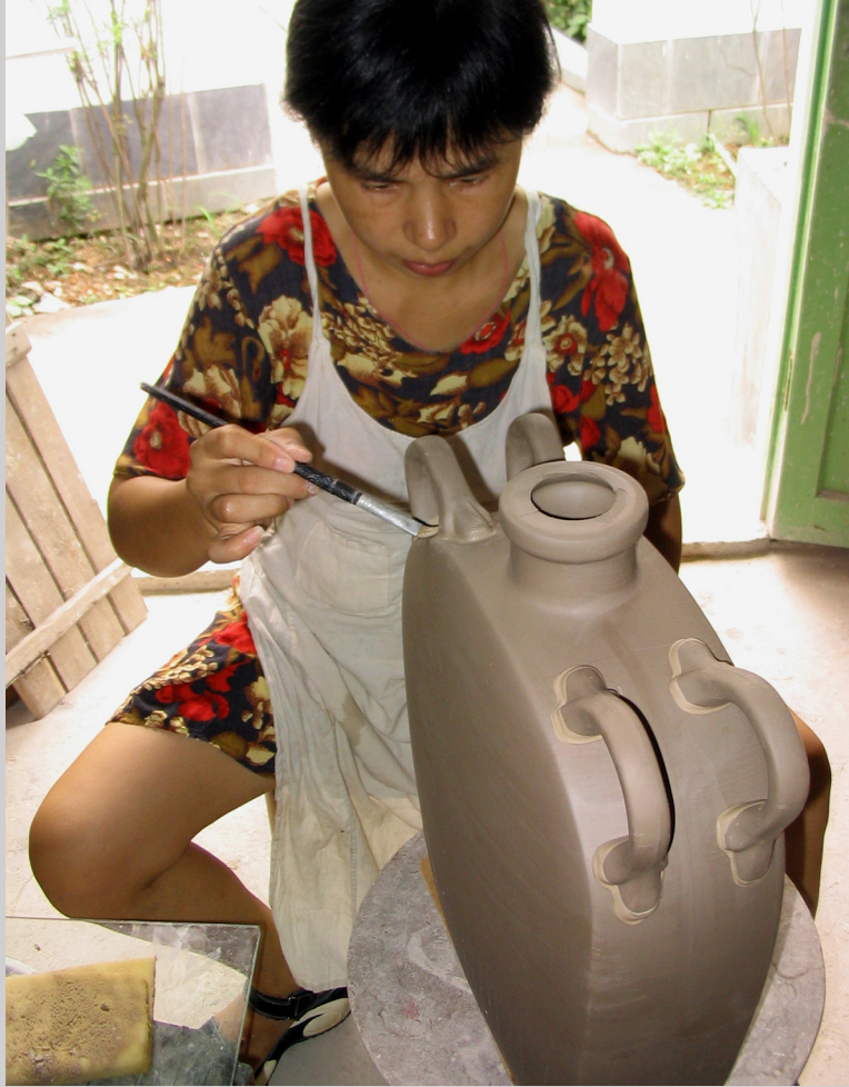
Figure 5.13e Applying cast handles with porcelain slip in Jingdezhen, China (photograph by Carol Ventura, 2004).
