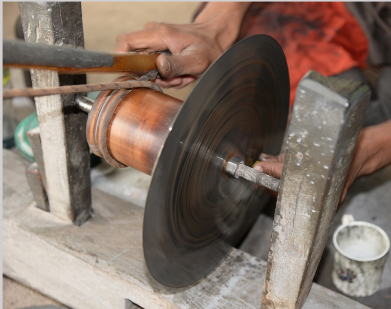
Figure 5.39f Shaping a dopped stone against a bow controlled abrasive wheel in Jaipur, India (photograph by Carol Ventura, 2016).
