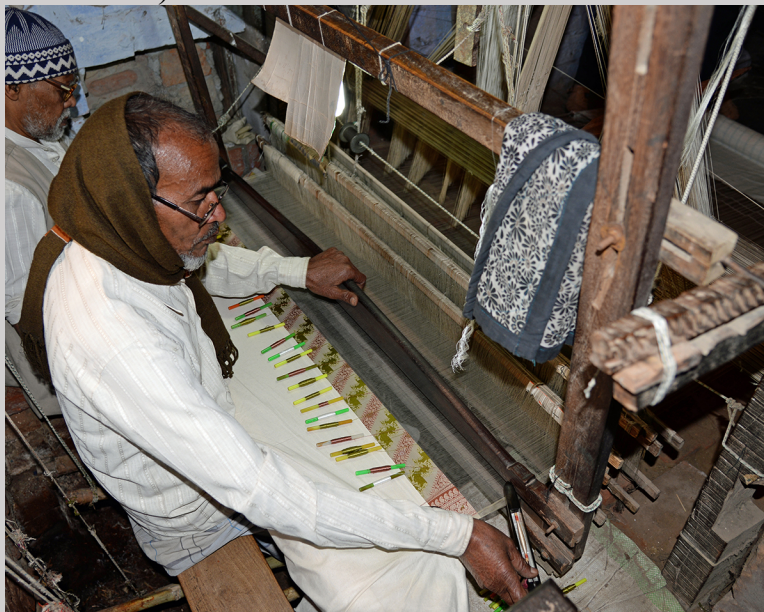
Figure 5.38k Inserting ground weft on a jacquard loom that was converted from a drawloom in Varanasi, India (photograph by Carol Ventura, 2016).
