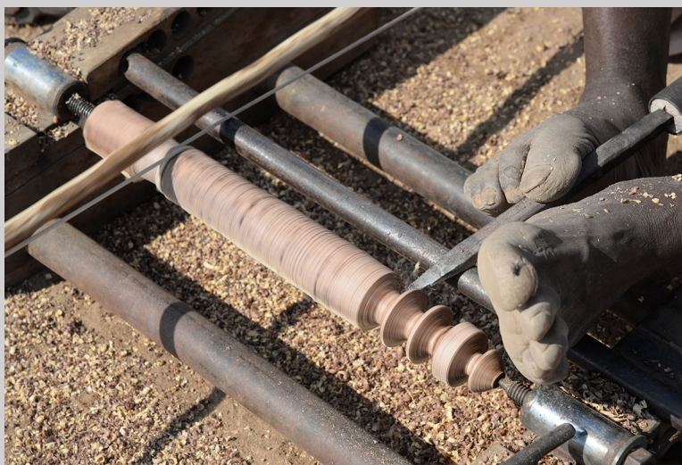
Figure 5.25a Bhachaya moves a bow back and forth with his right hand while operating a cutting tool with his left and his right foot to turn wood on a bow lathe in Nirona, Kutch, Gujarat, India (photograph by Carol Ventura, 2016).
