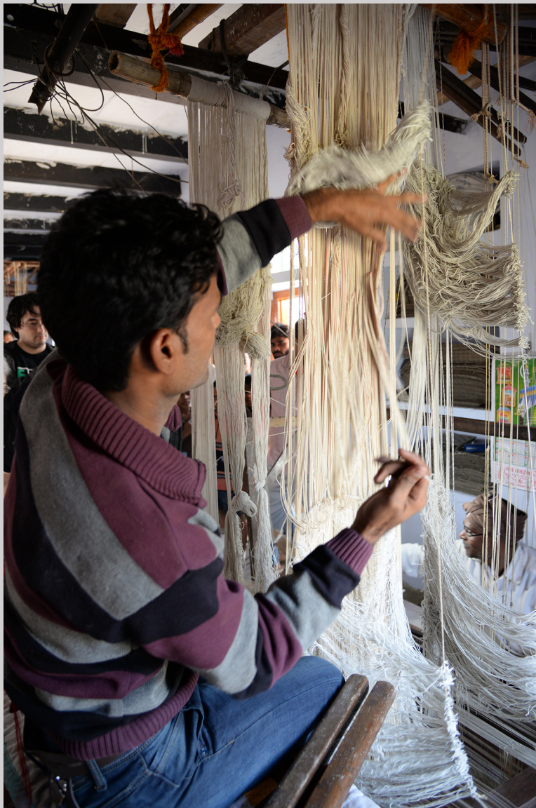
Figure 5.37a A knotted cord shows the “draw boy” which harnesses / shafts need to be raised to produce the next pattern shed in Cholapur, India
