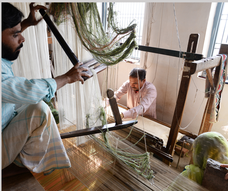
Figure 5.38c Belal raises drawcords with the lifting fork, then Shamin inserts silk pattern weft to produce voided velvet on their pit treadle drawloom in Cholapur, India (photograph by Carol Ventura, 2016).
