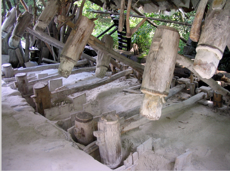
5.11b A water wheel drives the long, wooden axle. Wooden pegs (center back) trip the stone-tipped stampers as the axle rotates, Yaoli, China (photograph by Carol Ventura, 2004).
