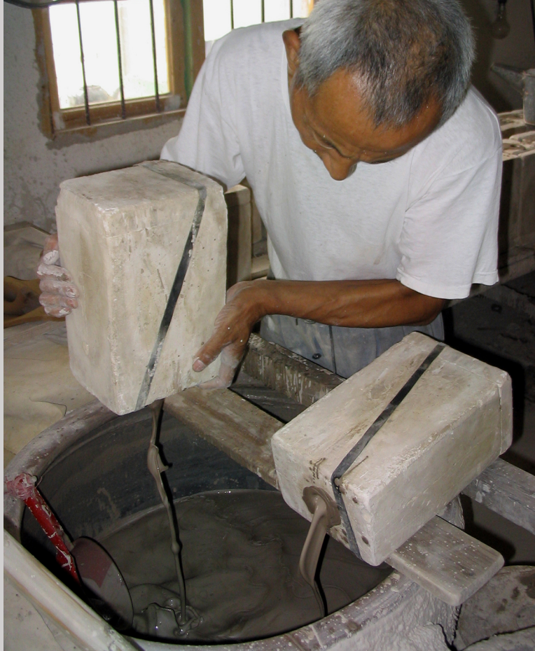
Figure 5.13b Pouring out porcelain slip to make a hollow form in Jingdezhen, China (photograph by Carol Ventura, 2004).
