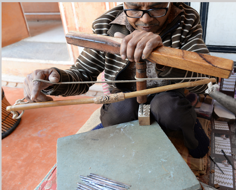
Figure 5.32c Using a bow drill and sharp metal bit to make holes in a block at the Anokhi Museum of Hand Printing, Jaipur, India (photograph by Carol Ventura, 2016).
