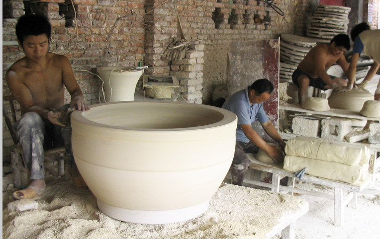
Figure 5.12i A pot is trimmed in the foreground, while clay is prepared for throwing in the middle ground and centered in the background at IAPFH in Jingdezhen, China (photograph by Carol Ventura, 2004).
