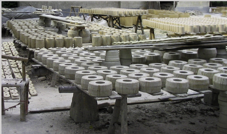
Figure 5.13c Slipware and plaster molds drying outside in Jingdezhen, China (photograph by Carol Ventura, 2004).
