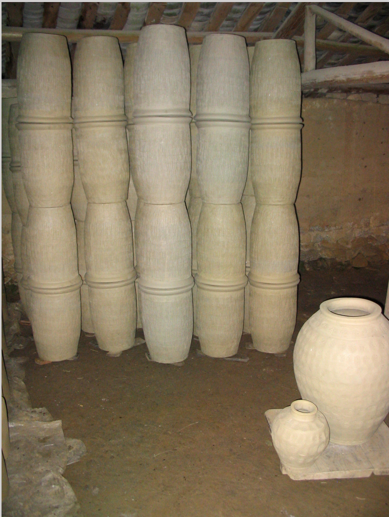
Figure 5.8e These stoneware vessels will be stacked base to base and rim to rim in the kiln just as they are stacked in a workshop storage room in
