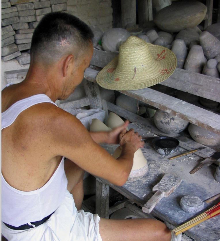
Figure 5.12b The leather-hard bowl is forced onto a smooth mold to standardize the bowl's size at the Jingdezhen Ceramic History Museum, China. Had it been placed on a decorative mold (as seen in Figure 5.12e), a pattern would have been transferred to the interior of the bowl (photograph by Carol Ventura, 2004).
