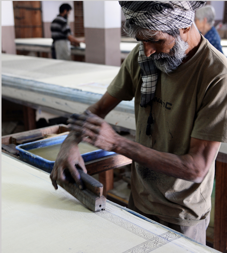
Figure 5.32f Printing a border on cotton cloth at the Dr. Ismail Mohmed Khatri Workshop in Bhuj, Gujarat, India (photograph by Carol Ventura, 2016).
