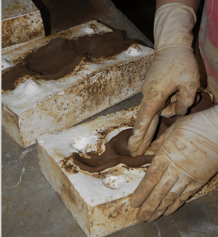
Figure 5.6b Terracotta is pressed into a two-piece plaster mold at the Art Ceramics and Lacquer Factory, Xian, China (photograph by Carol Ventura, 2013).
