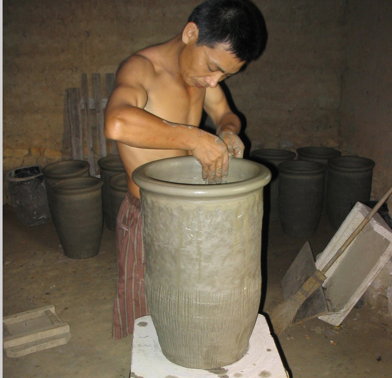
Figure 5.8c He then smooths the rim with a wet cloth in Tianbao, China (photograph by Carol Ventura, 2004).
