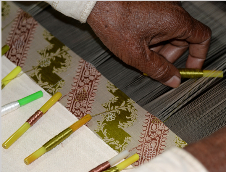
Figure 5.38m Inserting supplementary weft on a jacquard loom that was converted from a drawloom in Varanasi, India (photograph by Carol Ventura, 2016).
