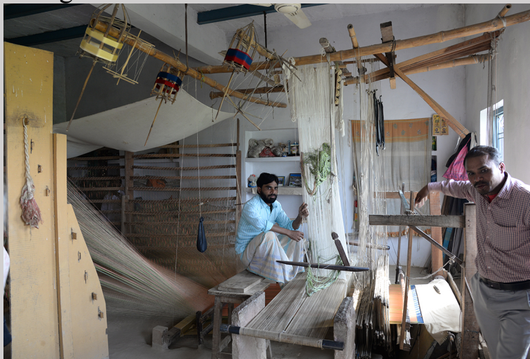
Figure 5.38a “Draw boy” Belal Ansari and his older brother, master weaver Rijvana Ansari, and their 21-harness pit treadle drawloom anchored to stone uprights buried in the floor in Cholapur, India (photograph by Carol Ventura, 2016).
